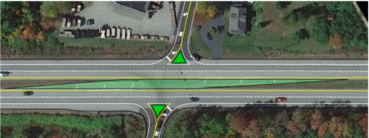
Figure 1. Graphic showing median closure at Beech Hill and Danville Corner Roads, taken from MaineDOT Safety Office presentation on HCL
